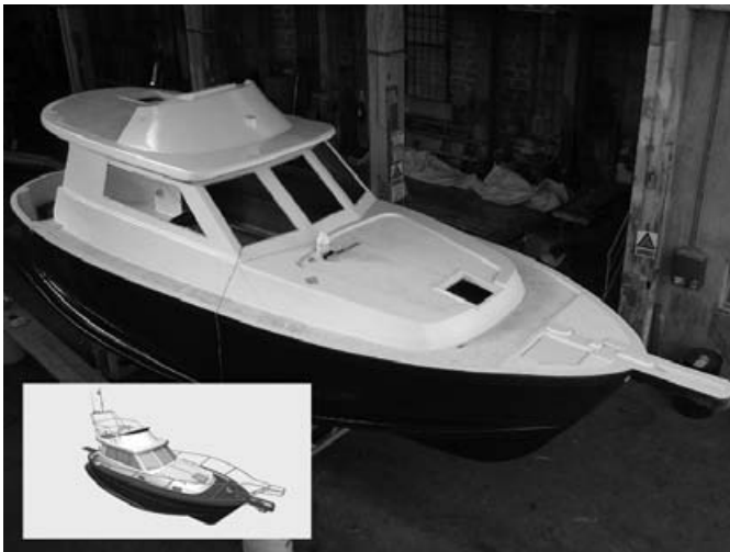
Figure 17: Prototype top view during outfitting (compared to virtual model to view)
