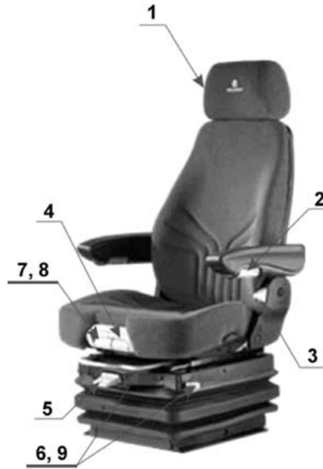
Figure 9. Tractor seat Grammer- ACTIMO XXL 12. 1 – Adjustable headrest, 2 – Foldable armrests adjustable height and angle, 3 – Adjustable seatback, 4 – Adjustable seat angle, 5 – Height adjustment, 6 – Fore/aft adjustment, 7 – Variable seat length, 8 – Adjustable airbag, 9 – longitudinal muffler
