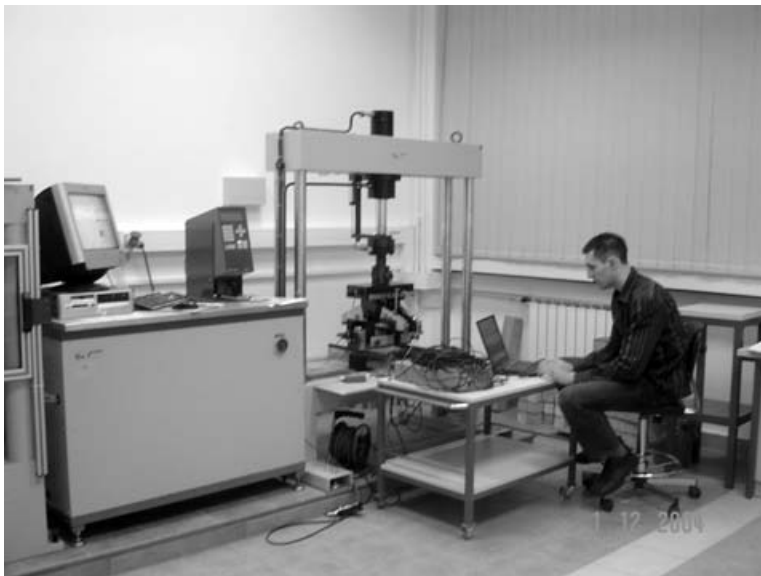
Figure 3: Testing of mechanical properties of ultra-high strength concrete in the laboratory of the Department of Materials, Faculty of Civil Engineering in Zagreb
