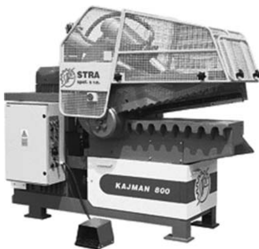
Figure 2: Hidraulically-driven alligator shear (STRA spol.sr.o., 2005)
