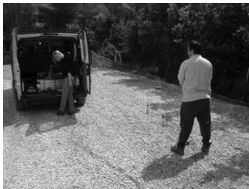
Figure 8: Quality control of soil improvement by the Spectral Analysis of Surface Waves method
